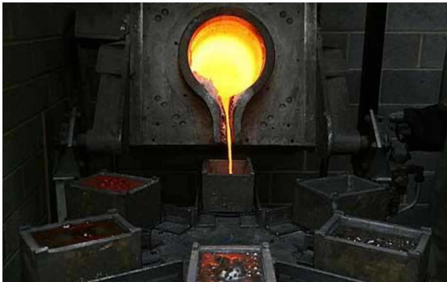
Liquid gold: Gold is poured from the induction kiln Photo: JULIAN SIMMONDS
